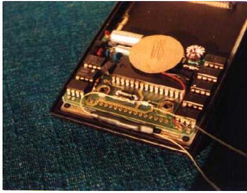
Close up view of my HP 41C board, showing the connection of the TONE interface. A series resistor, used as a limited short-circuit and ESD protection, was inside the heat-shrunk tube.
