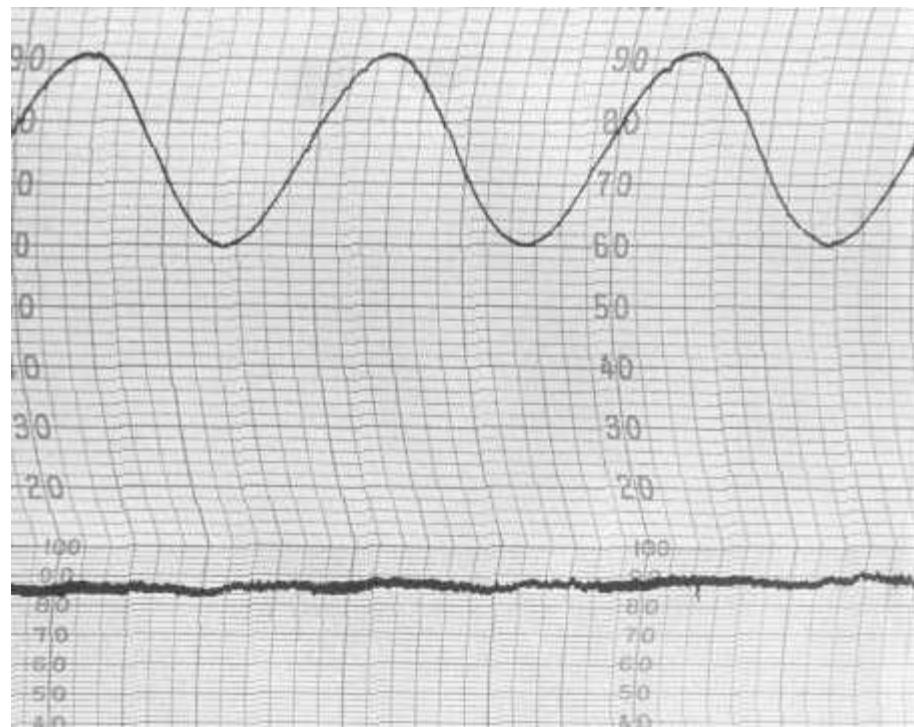
The level of environmental control that we could obtain within the chambers using the HP9100 calculator was impressive. The graph above is the output of a mechanical hydrothermograph. This specific data was an early test run to demonstrate the chambers' capabilities over a two-week test run (only three days are visible in the photo above).
