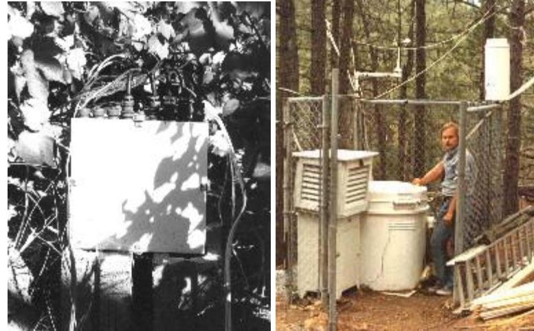
Remote telemetry stations were designed and constructed so that up to 16 sensors per station could transmit abiotic (weather) information back to the HP9100A calculator. The two principal research efforts at the time concerned phytophagous cotton insects and bark beetle infestations in the Lincoln Forest.
