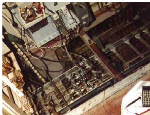
Using the HP 41C to calibrate an analog-to-digital converter, that monitors a compressor in a computer-controlled CO<sub>2</sub> production plant.
