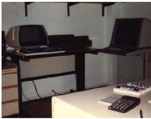
My HP 41C helped in the design of a custom interface prototype (white breadboard). A Data General Dasher terminal, a plotter, and a Tektronix graphics terminal (with storage CRT) are also shown (left to right).
