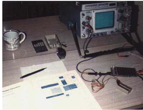
Trying to peek (with poor results) into my HP25. Note the Tektronix 465 oscilloscope with a DM 44 multimeter optional feature in top.
