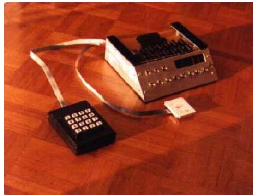
A homebrew RCA 1802 microprocessor (COSMAC) prototype system, used to "read" TONE commands from my HP 41C.
