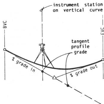
When the station that is occupied by the instrument is within a vertical curve, the elevation that is input as profile grade is the elevation of the **vertical tangent** at the instrument station.
