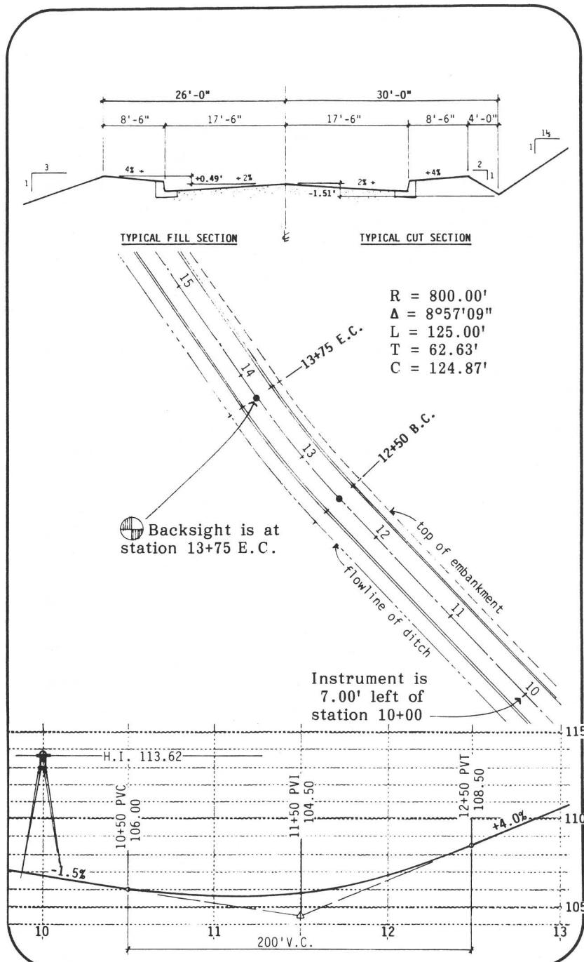
Before you begin input of the alignment information, take a moment to calculate the cut and fill factors. This is simply the difference in elevation between the finish profile grade and the hinge point you are staking to. If for instance, you were staking to the back of a bench in a cut section, this could be a difference of 20 or more feet.
