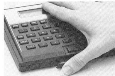
To remove the ROM module, use your fingernails to grasp the lip on the bottom of the front edge of the module and pull the module straight out of the port. Install a blank module in the port to protect the contacts inside.
