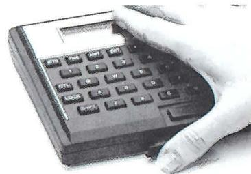
To remove the module, grasp the lip on the bottom of the front edge of the module and pull the module straight out of the port. Install a blank module in the port to protect the contacts.
