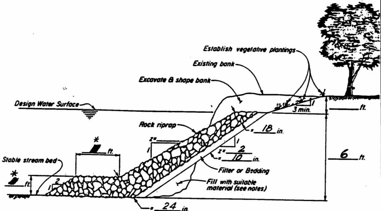
\* See Alternate TYPICAL CROSS-SECTION Detail (not to scale)
