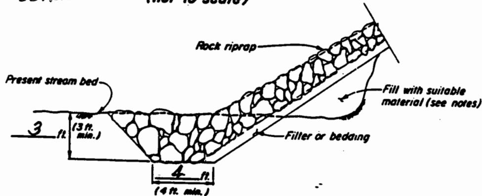
ALTERNATE TOE CROSS-SECTION (not to scale)
